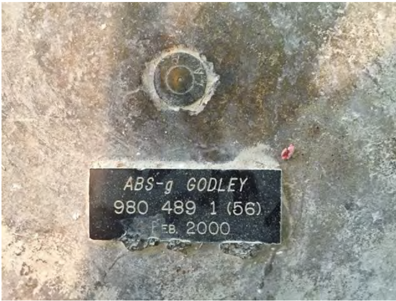
The Godley head floor plaque in Feb 2000 (156) indicates a “0 m” value 2 \mu\text{Gal} higher than the final Feb 2000 value at 1 m.
